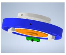
5) Install tool over chuck body until it is resting on riser blocks
